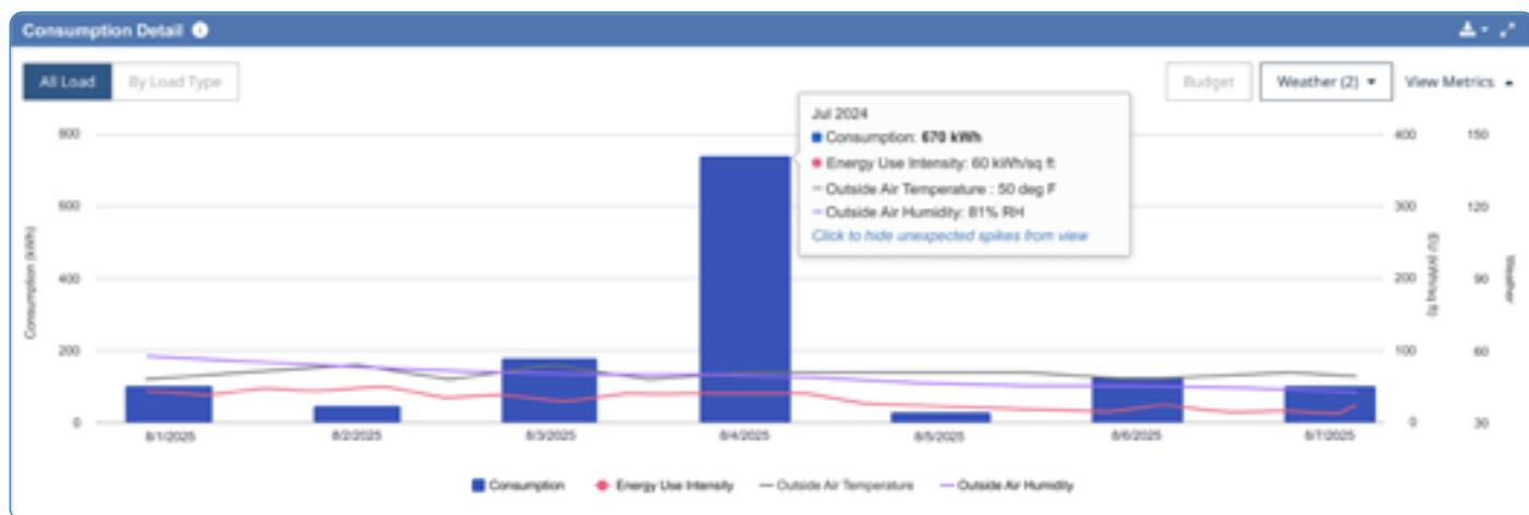
*Report reflects a sudden spike in energy consumption, despite stable ambient conditions as indicated by the overlaid weather data. This suggests a possible equipment fault.*
