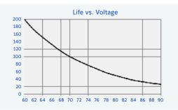
Effects of application voltage vs. rated voltage
