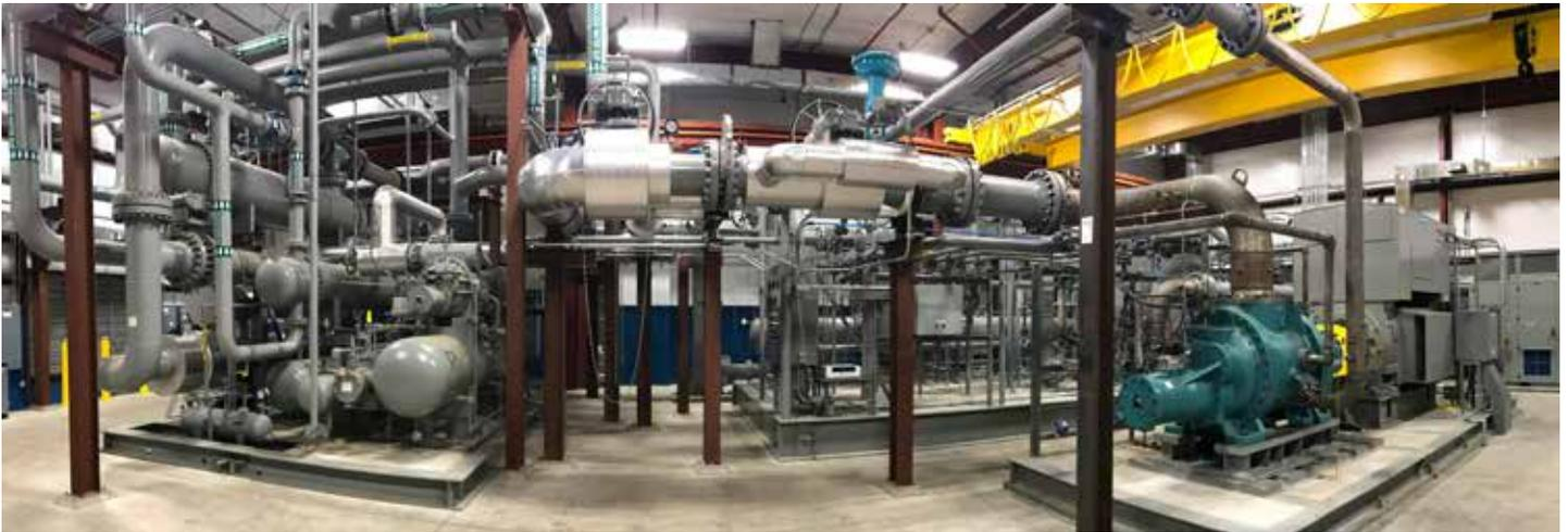
Our new, high-pressure, variable speed, Screw Compressor Test Stand is one of the largest, most sophisticated test stands in the screw compressor industry, and is a significant addition to our existing lab.
